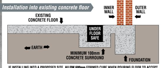
IF INSTALLING INTO A PROPOSED SITE, **ALLOW 600mm** FORMED CUBE WHEN POURING FLOOR TO ACCEPT FLOORSAFE, WHEN HOUSE IS UP TO LOCKUP STAGE, THEN INSTALL IN CONCRETE IN IMMEDIATE AREA.
