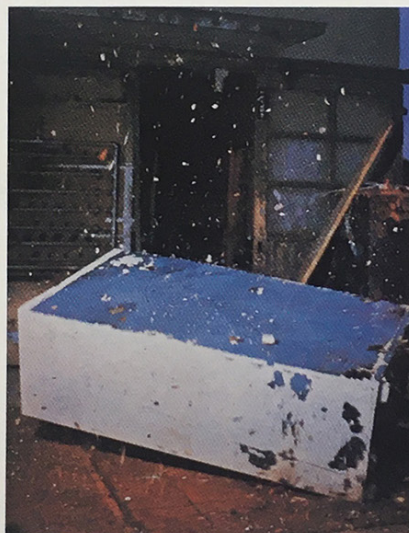
Cabinet dropped 9 metres onto bricks laid on concrete flooring.
