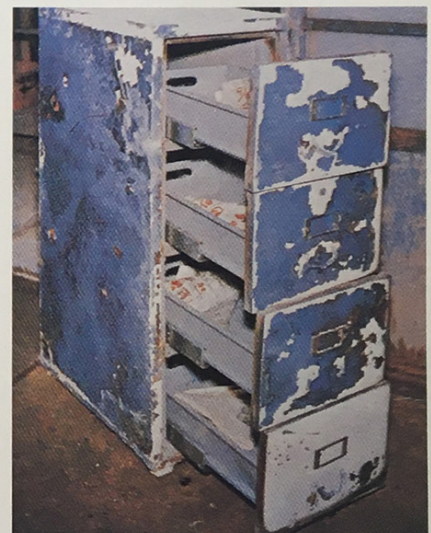
Tests proved high efficiency of fire resistance. Printed matter remained legible after test.
